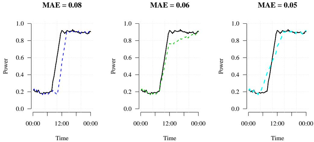
**Figure 4.1:** Examples of different types of ramp forecast error. Actual power is shown as solid black lines, forecasts are colored dashed lines. From left to right: phase or timing error, level error and ramp rate error. The mean absolute error (MAE) for each forecast is shown above the plots. Despite being the only forecast that correctly predicts the ramp rate and duration, the forecast with a phase error has the largest MAE.
