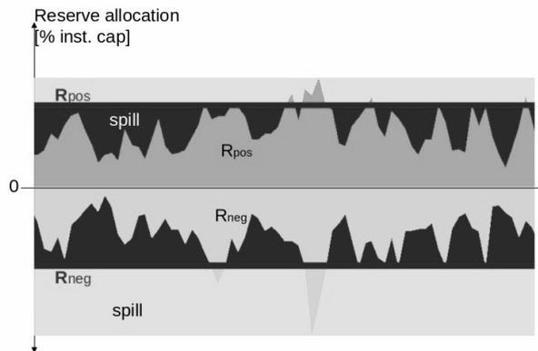
**Figure 5.7:** Illustration of the “reserve allocation dilemma” of costly spill versus covering all possible ramping events. Here,  $R_{pos}$  is the dynamic positive reserve,  $R_{neg}$  is the dynamic negative Reserve, the upper linear borders  $R_{pos}$  and  $R_{neg}$  are the static reserve allocation, the black area and the outer light gray areas are the spill for the dynamic and static allocation of reserves, respectively.
