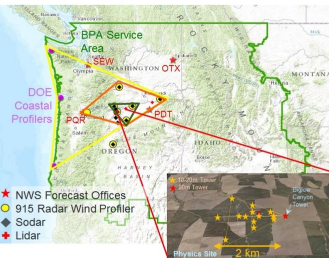
Figure 1: The Instrumentation of the Second Wind Forecast Improvement Project (WIP2), in the Northwest of the USA. Source: Joel Clain.
