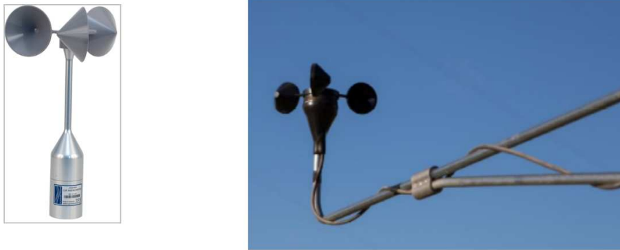
Figure 2.4: MEASNET certified cup anemometer from Campbell Scientific and a cup anemometer 40C from RNRG.
