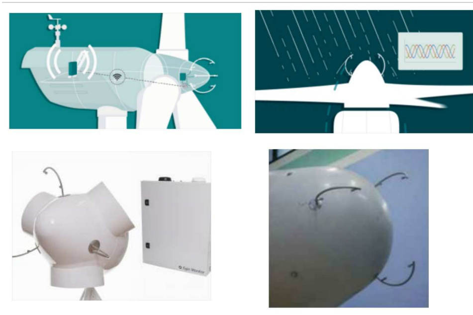
Figure 2.6: Ultra-sonic anemometer spinner technology iSpin from ROMO Wind as schematic and also an example of a nacelle top mounted from METEK (bottom right).
