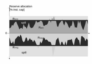
**Figure 5.7:** Illustration of the "reserve allocation dilemma" of costly spill versus covering all possible ramping events. Here,  $R_{pos}$  is the dynamic positive reserve,  $R_{neg}$  is the dynamic negative Reserve, the upper linear borders  $R_{pos}$  and  $R_{neg}$  are the static reserve allocation, the black area and the outer light gray areas are the spill for the dynamic and static allocation of reserves, respectively.
