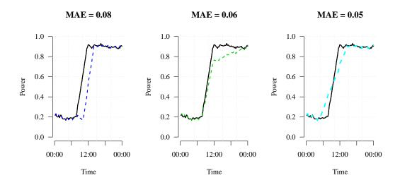
**Figure 4.1:** Examples of different types of ramp forecast error. Actual power is shown as solid black lines, forecasts are colored dashed lines. From left to right: phase or timing error, level error and ramp rate error. The mean absolute error (MAE) for each forecast is shown above the plots. Despite being the only forecast the correctly predict the ramp rate and duration, the forecast with a phase error has the largest MAE.
